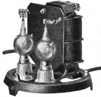
RECTIGON WITH COVER REMOVED, SHOWING ALL PARTS
